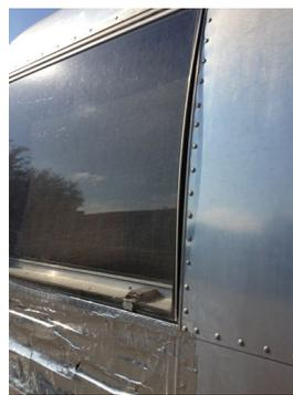
not exactly leaving gaps where water can get in. In addition, the rubber seals around all of the windows and door are dried
